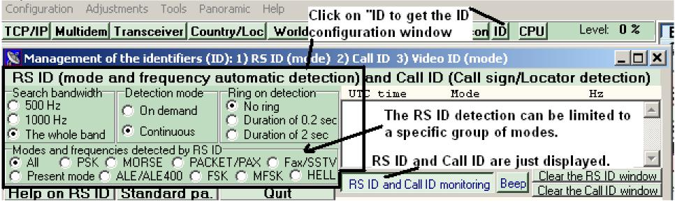
Buttons to push to start automatic decoding or to transmit a RS ID
