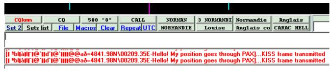
Here is part of the Multipsk screen, after reception of the position transmitted by the other Multipsk (previous screen) in PAX or PAX2 (PAX2 here) and repetition towards UI-VIEW in Kiss mode:
