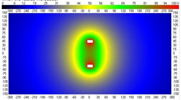
It can be observed that, from left to right on the axis, the induced potential increases up to U0 at the center of the lens and then decreases from U0.
