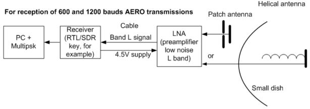
Necessary hardware with a Patch antenna:
